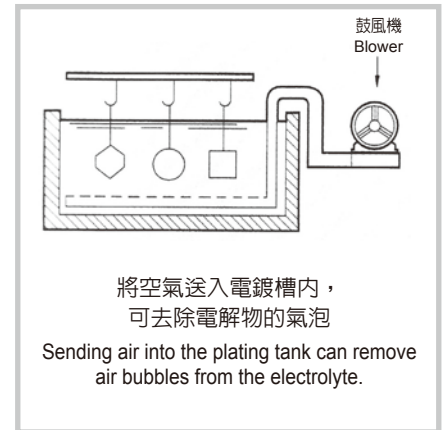
電鍍槽 Plating tank
